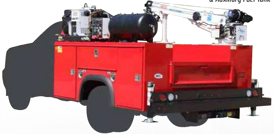
Crane, Air Compressor, Engine & Auxillary Fuel Tank
