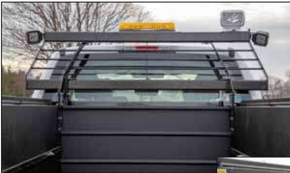
Cab Rack with Strobe Light, Spot Light, Work Lights, Durabed Lining in Loadspace & E-Track
