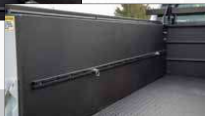
Cab Rack with Strobe Light, Spot Light, Work Lights, Durabed Lining in Loadspace & E-Track
