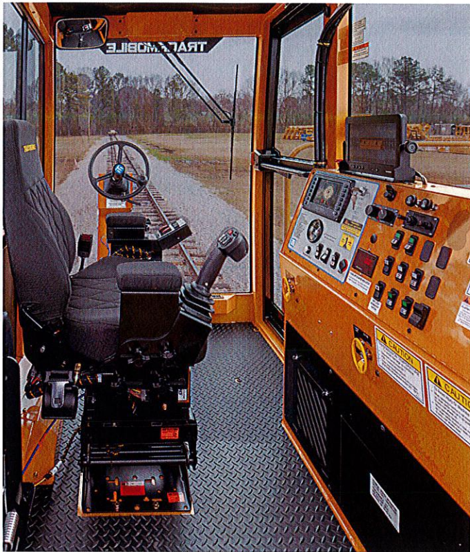
Titan control panel and operational controls.
