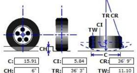
С - Curb Contact Length: 15.91 - Curb Clearance Increment: CI 5.84 CR - Curb Clearance Radius: 36'9" CH - Curb Height: 6" - Turning Radius: 36'3" TR TW - Tire Width: 11.10
