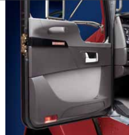
Available in Diamond (right) and Splendor (above) upholstery, Kenworth's new door pad presents a soft, durable, low-gloss luxurious finish you might associate with the finest automobiles. The new door pad design positions the window, door lock and mirror controls for easy touch access.
