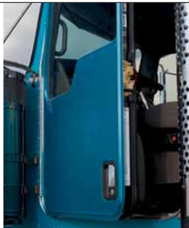
Thick bulkhead-type doors hang on continuous stainless steel piano hinges – not typical automotive hinges – and fit snugly to become an integral part of the cab structure – another reason Kenworth trucks bring more at resale than just about any other make you can name.
