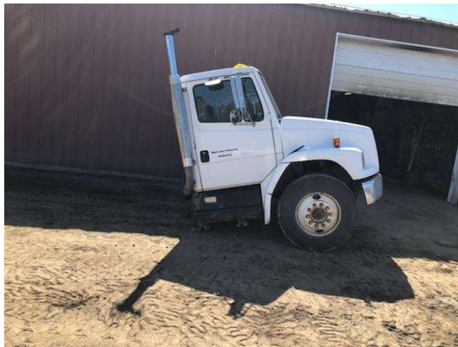
Figure 2. Frame of 1993 Freightliner cut in half.
