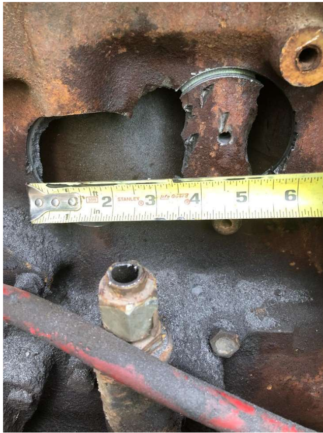
Figure 7. Hole drilled in 1994 Ford engine block.
