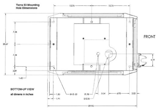
Figure 1: Terra x3 mounting-hole locations, in inches.
