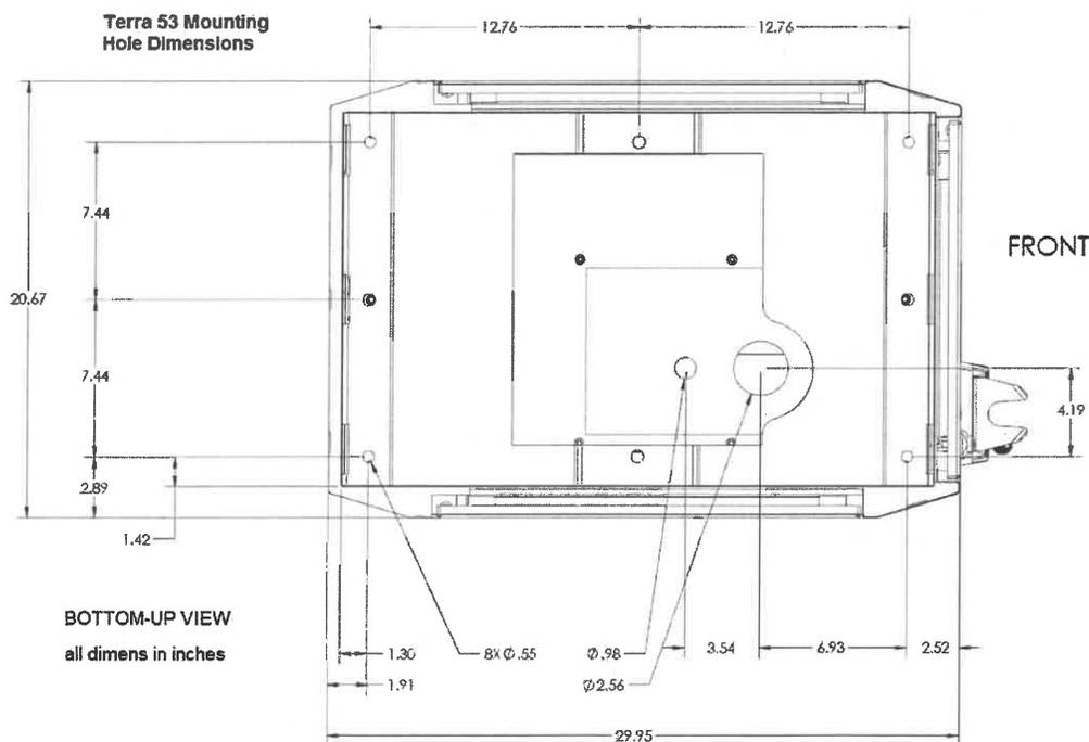
Figure 1: Terra x3 mounting-hole locations, in inches.
