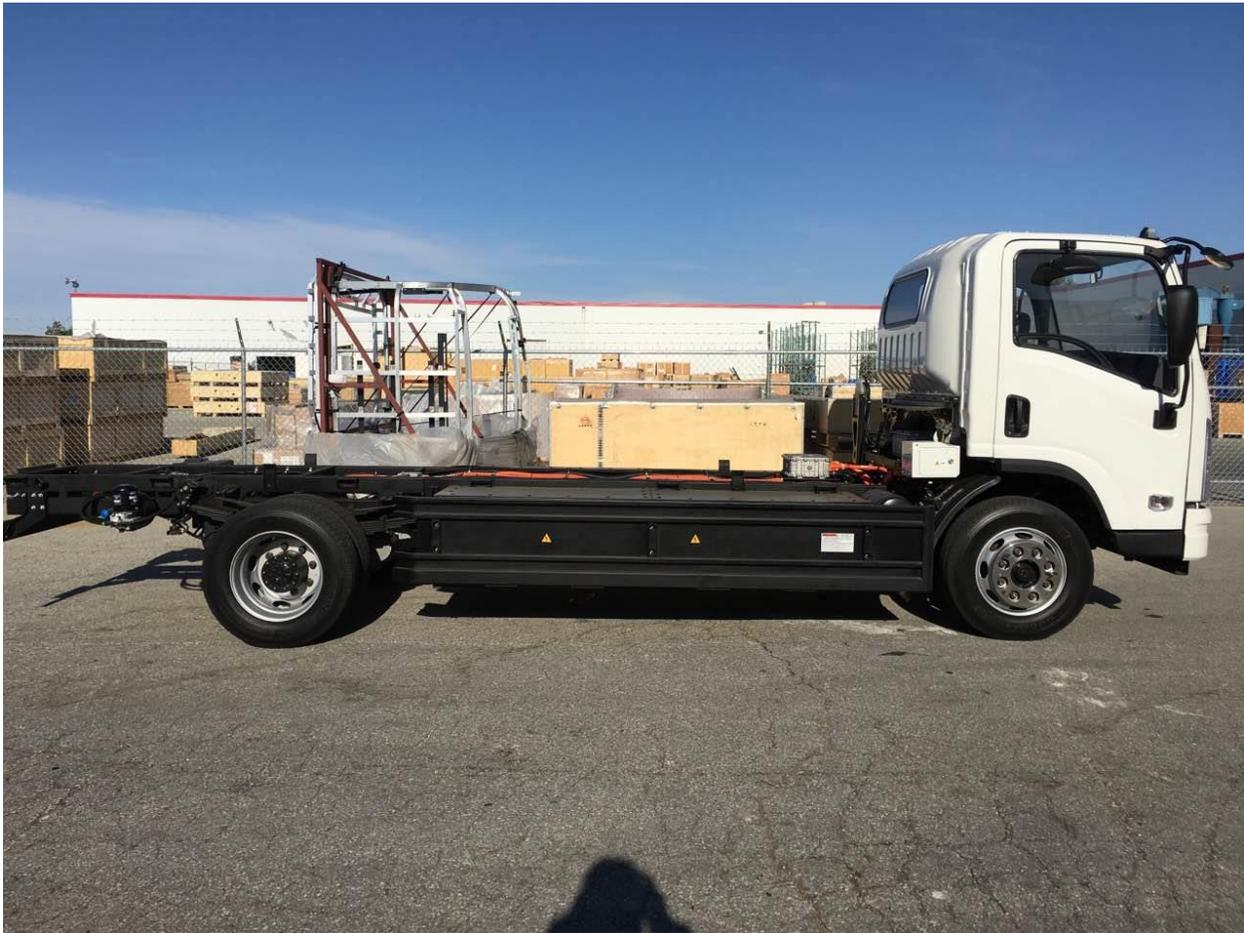
BYD recommends using a 20 ft box from Supreme Corporation with MDL20 liftgate. The liftgate will have cart stops. The quote below shows approximate specifications, which will be finalized with the customer.
