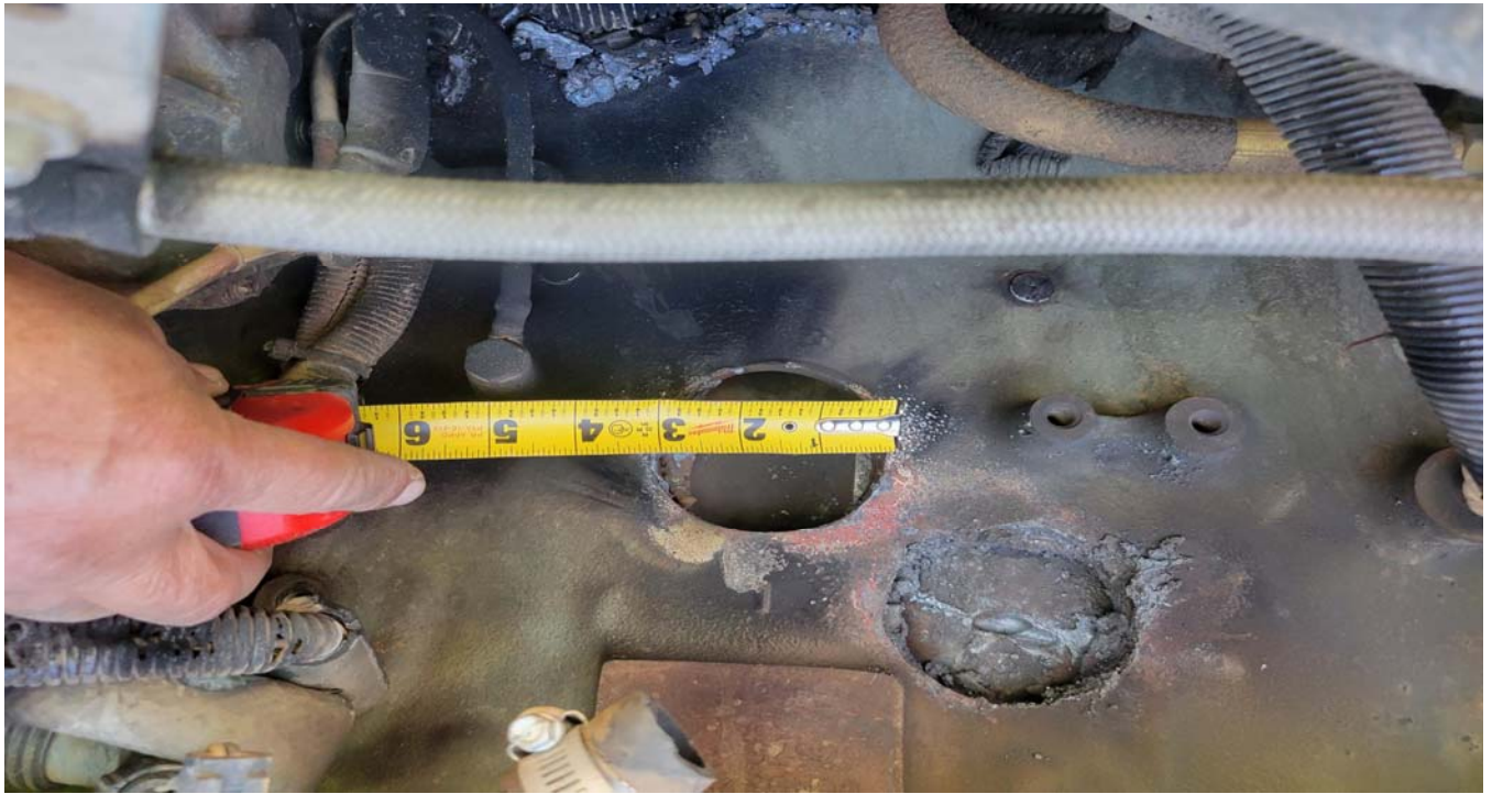
Photo No. 13 Dismantle and Scrappage – 3” Hole in Engine Block Close-Up
