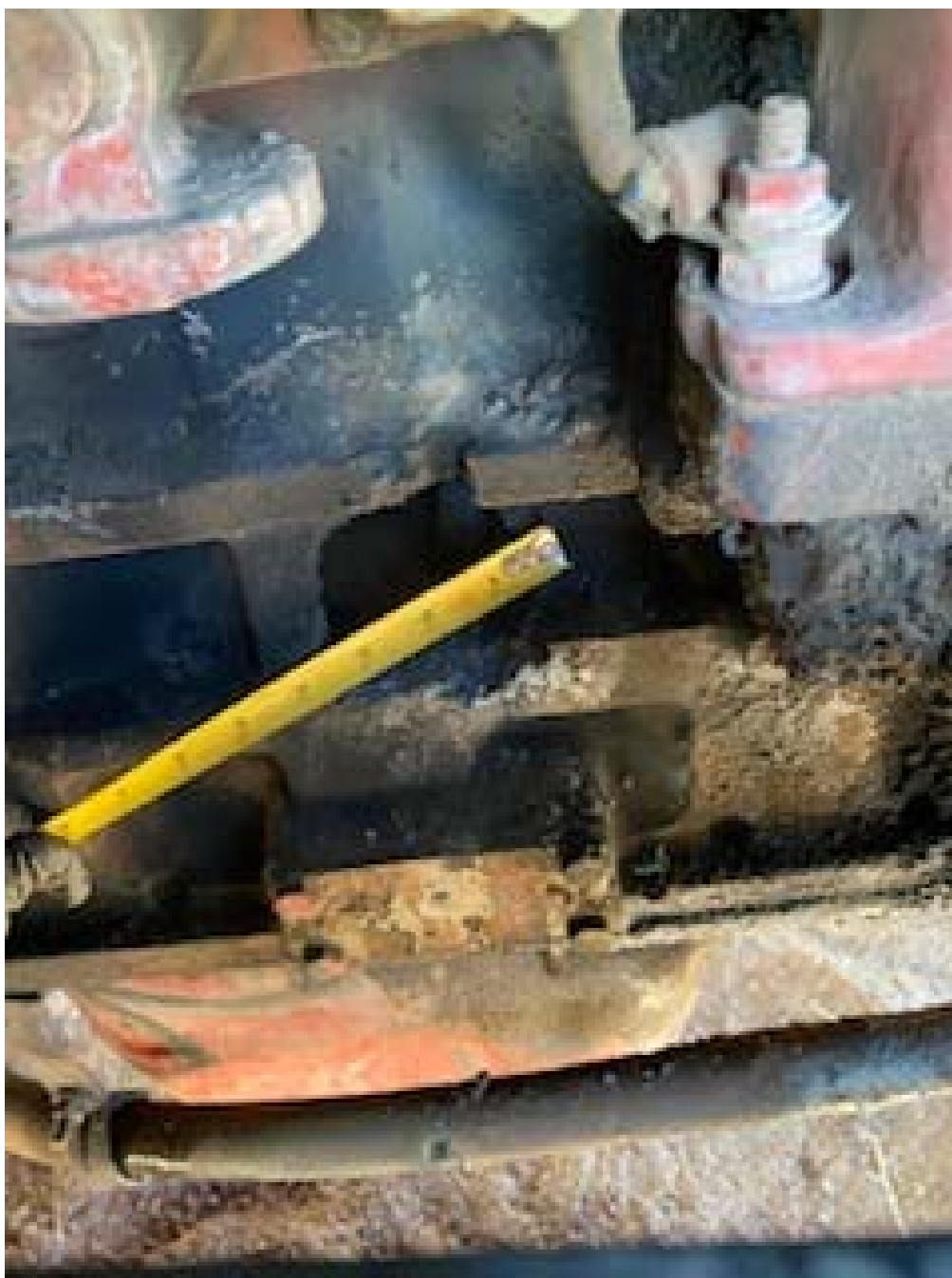
Photo No. 12 Dismantle and Scrappage – 3” Hole in Engine Block
