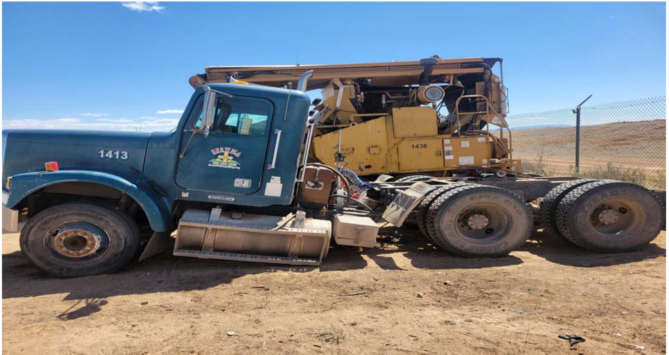
Photo No. 11 Dismantle and Scrappage – Chassis Rail Cut Overall View
