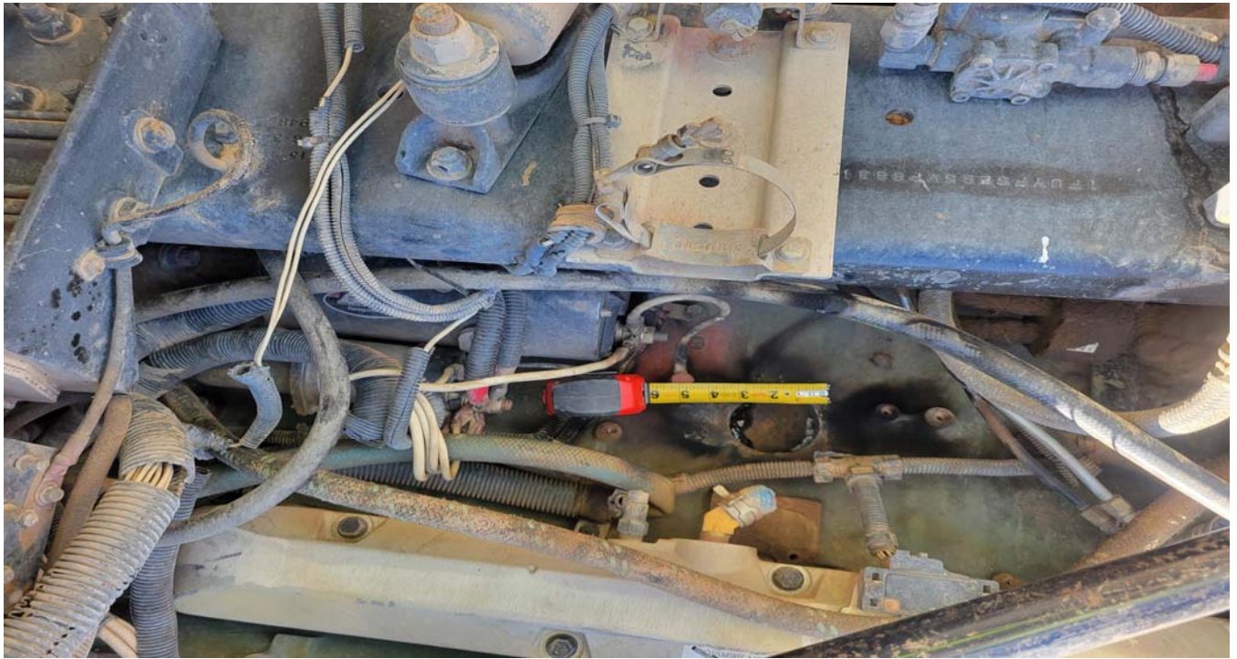
Photo No. 12 Dismantle and Scrappage – 3” Hole in Engine Block
