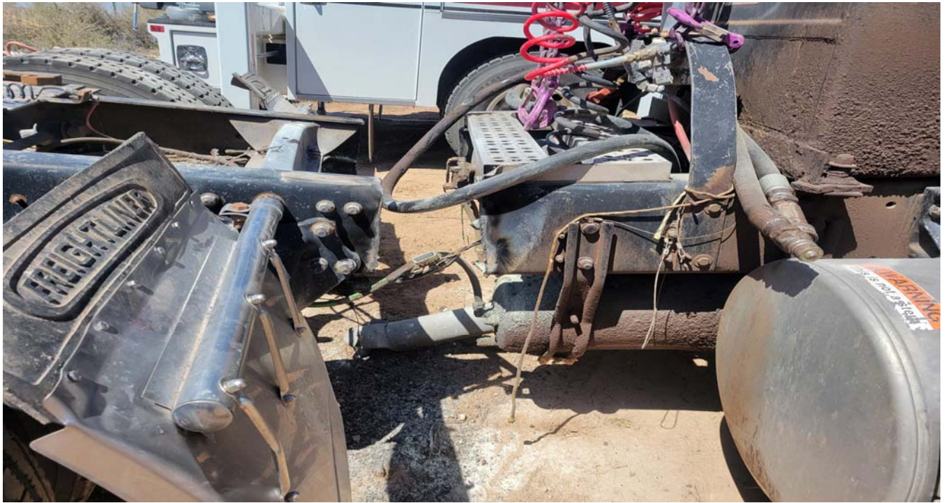
Photo No. 10 Dismantle and Scrappage – Chassis Rail Cut Close-Up
