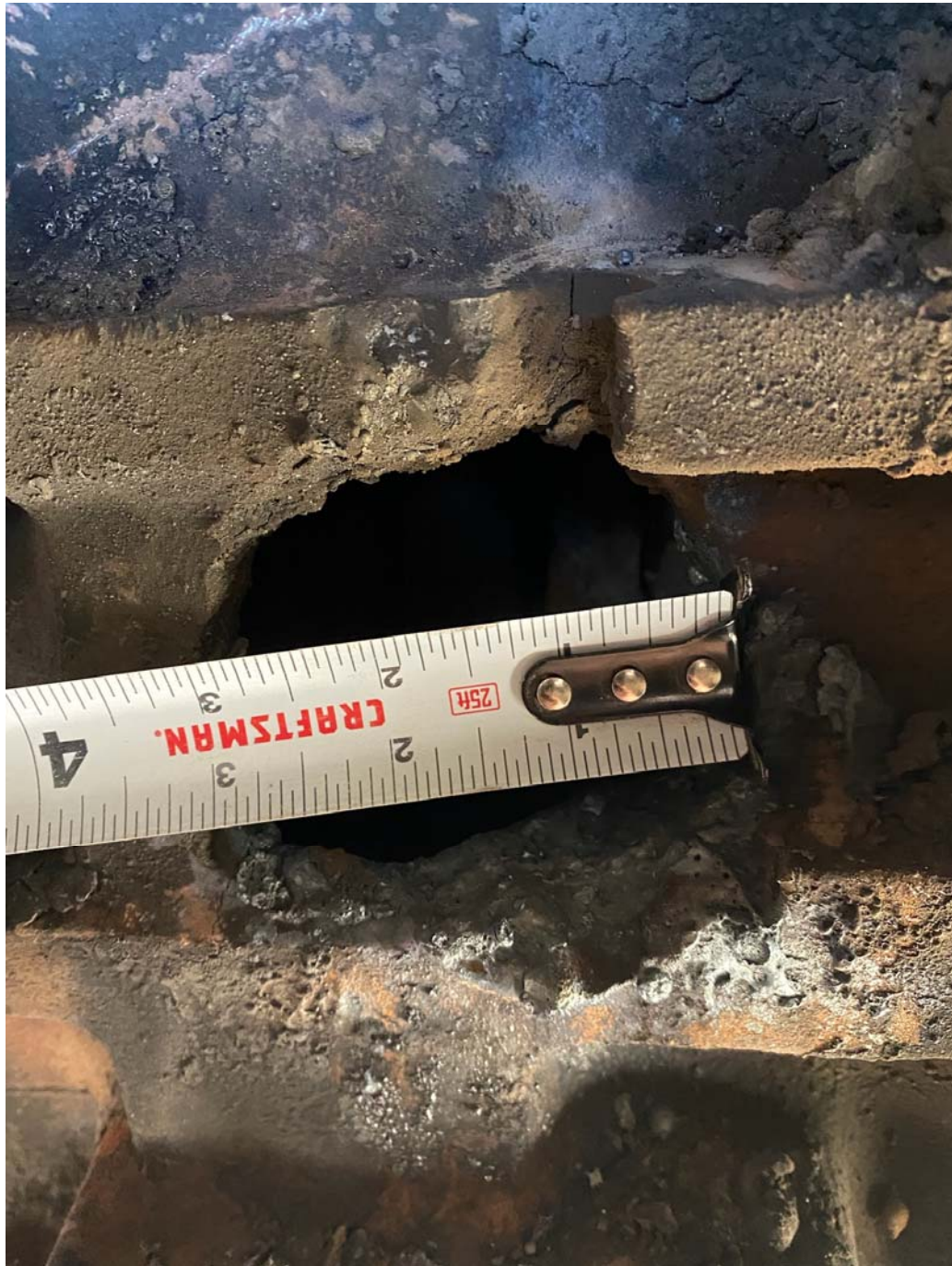
Photo No. 13 Dismantle and Scrappage – 3” Hole in Engine Block Close-Up
