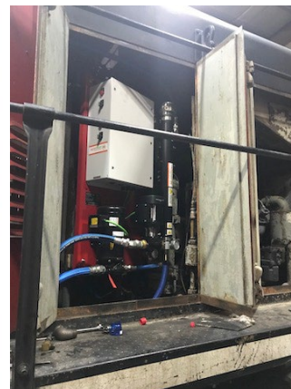
Locomotive idle-reduction technology such as Auxiliary Power Units (APU) and Automatic Engine Shutdown/Start up (AESS) allow locomotives to reduce time spent idling, thus reducing fuel consumption and emissions. APUs act as a small engine, warming and circulating coolant and oil, allowing the main locomotive to shut down while retaining the ability to restart immediately. (Pictured right) An APU installed on one of the five locomotive grant projects funded.
